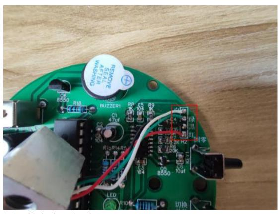
7: Assemble the electronic scale First fix it on the board with two short screws and copper pillars;
